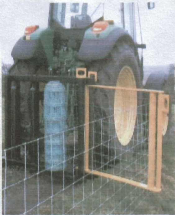
The Quickfencer boosts safety and makes for quicker working when erecting wire fencing.
